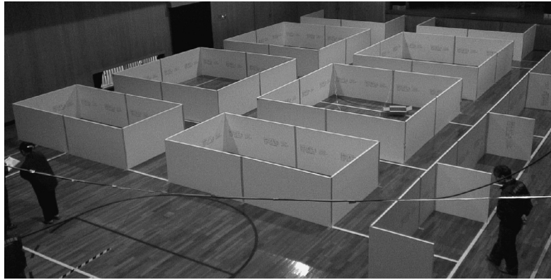
Fig. 8. Overview of a model simulating Kyoto city, which has a checkerboard design of streets and avenues. The walls are foam sheets.
